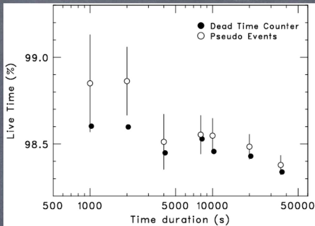
Both the dead-time in the electronics and the signal loss due to the chance coincidence can be corrected by counting “the pseudo events” which are periodically produced in the onboard electronics. The time interval when the telemetry saturation has occurred are already excluded from the GTI of cleaned event files.
