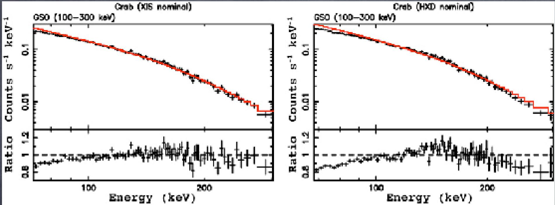
The residuals of the Crab fitting are less than 10% at 70–200 keV, but significantly larger outside that energy range. We are now investigating various parameters in the MC simulation. We recommend all users to verify your spectrum by creating “the Crab ratio” before trying to fit the spectrum in XSPEC.
