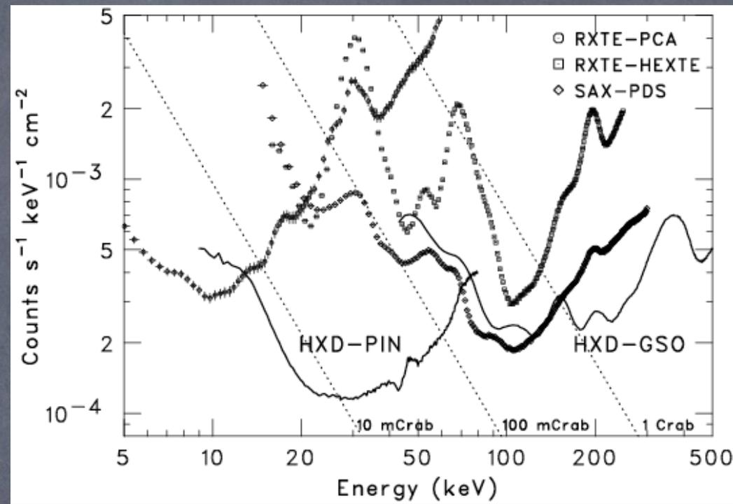
By fully utilizing the anti-coincidence with the active shield, the lowest background level (per the effective area) has been achieved in HXD-PIN.
