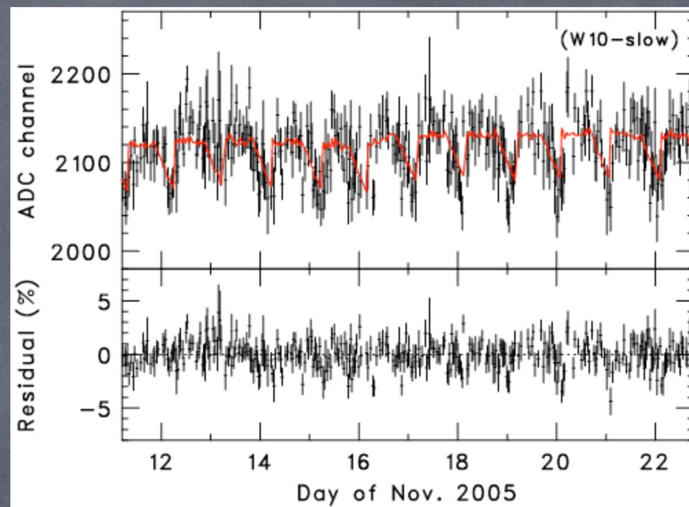
The long-term and short-term gain variations are observed. The former is caused by the degradation of the PMT gain, while the latter is due to both of the temperature dependence of the GSO light-yield and aging effect in PMT gain during the SAA.
