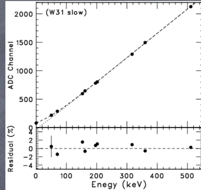
In-orbit GSO energy scale is derived by use of the EC-decay peaks in the background spectrum, together with the 511 keV line. Since a significant non-linearity appears below 100 keV, the uncertainties become larger in this energy range.
