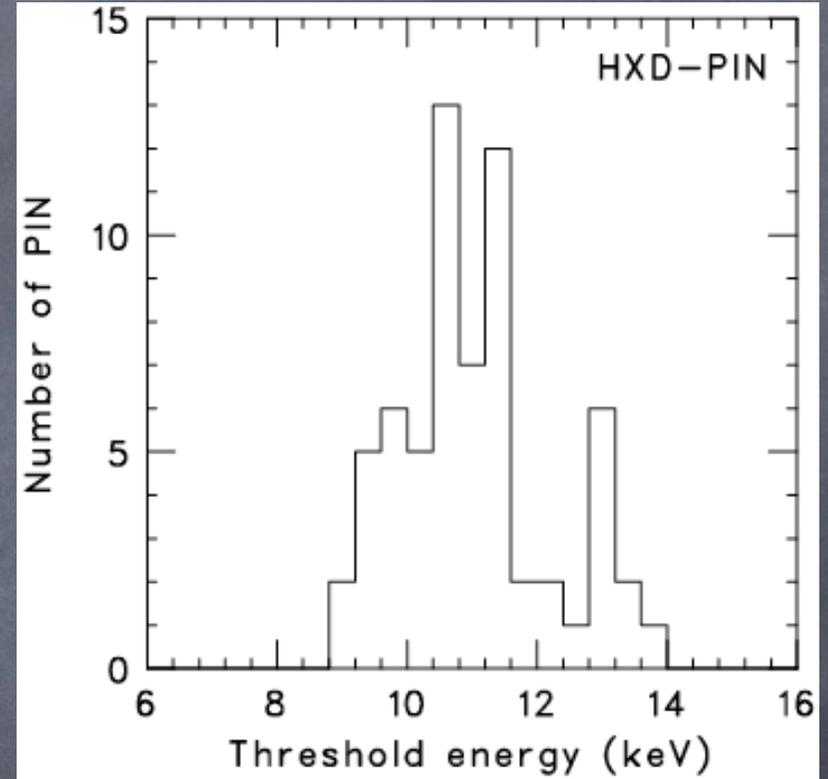
Noise events (thermal and electrical) are rejected by both of onboard and software cuts, which are individually optimized for 64 PIN diodes. Resultant lower threshold energy varies from 9-14 keV.
